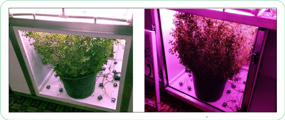
Figure 3. General view of the gas exchange chamber during the day and at night with plants of Ligustrum vulgare L. Source: created by the authors
